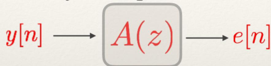
Filter is stable - error signal is white
