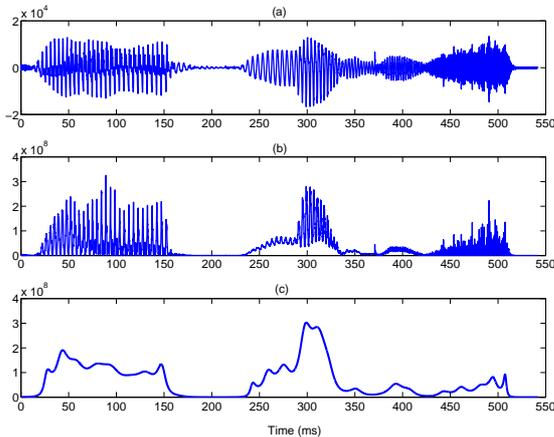
**Fig. 1.** Illustration of the all-pole modelling property of FDLP. (a) a portion of the speech signal, (b) its temporal envelope, and (c) all pole model obtained using FDLP.
