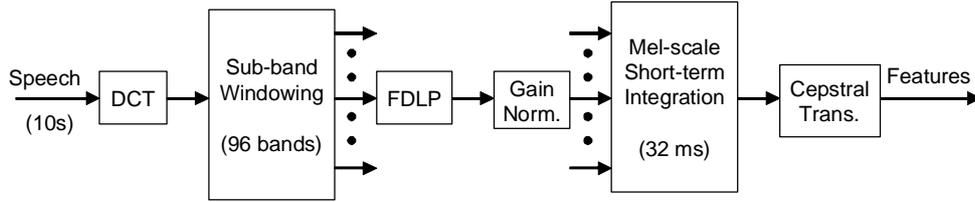
**Fig. 2.** Block schematic of the proposed feature extraction.
