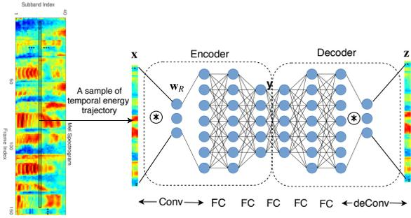
Figure 1: Block diagram of temporal modulation filter learning using CAE from spectrograms.
